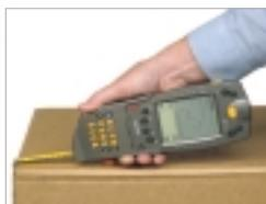
Simply measure the three axes using the TallyMan DWM 1828's in-built tape measure for automatic capture on the Symbol pocket computer
