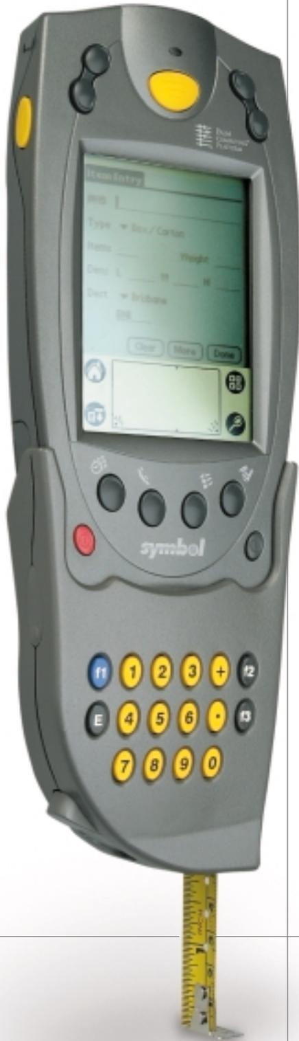
The TallyMan DWM 1828 is a groundbreaking new accessory that enables dimensional weight data (dim.wt) to be captured on Symbol Technologies' SPT 1700, 1800 and PPT 2800 hand-held pocket computers. The TallyMan DWM 1828 is compact and portable, and attaches direct to the pocket computers.
